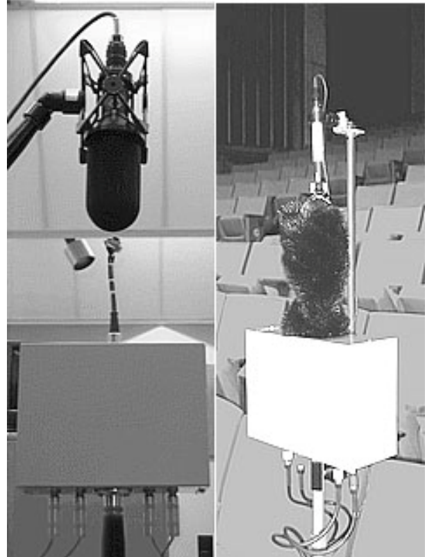
Figure 5 – Soundfield SPS422B and experimental mic without its windscreen (left). Experimental mic with windscreen and Core Sound TetraMic on the dual mount (right).
