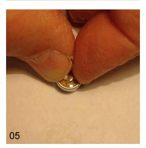
01-05. The electret microphone capsules are manufactured as 2-terminal devices. There is an FET (field-effect transistor) inside the capsule, one terminal of which is connected to the case of the capsule externally. The first step is to cut that connection and make the capsule a 3-terminal device. This greatly increases the dynamic range and the clipping level of the microphone.
