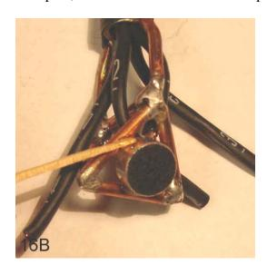
16B. Roll the epoxy with the toothpick into the valley formed by the capsule and its supporting wire. Do this for all 3 edges.
