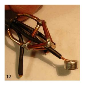
12. Place your thumb on the face of the capsule and index finger on the terminals. Gently bend the wires so the capsule is almost parallel with face 1 of the tetrahedral without bending their connections to the capsule terminals.
