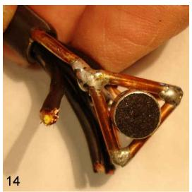
14. Before the capsule is seated on the tetrahedral, gently press the number 1 pair against one of the vertical sides of the U-frame. Do not pull tight; the shield wire and terminal 3 of the microphone capsule are fragile. If needed, push the number 1 pair from the bottom of the pipe for some slack. Capsule 1 is the LFU (left-front-up) capsule.
