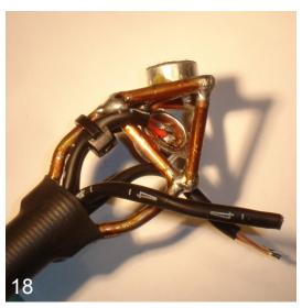
18. Capsule 2 in place with the epoxy set for a half hour. Before adding the tie-wrap, be certain the pairs lie next to the copper wire of the U-frame. If not, push more wire up from the bottom of the pipe. Pull the tie-wrap just snug.
