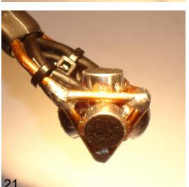
20. There is not much space for pair 4. Be sure the epoxy for the first 3 capsules is well set before continuing to the final capsule. Note the wire routing of the number 4 pair.
