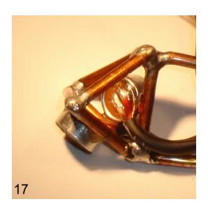
17. Capsule 2. Note the final routing of wire pair 2. Capsule 2 is the RFD (right-front-down) capsule.
