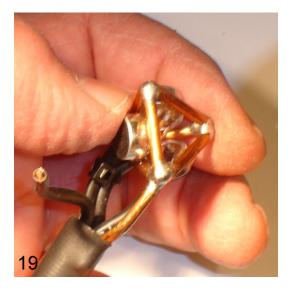
19. Capsule number 3 faces *down*. Capsule 3 is the LBD (left-back-down) capsule. This is the ambisonic a-format order, not a clockwise rotational order. Also, note the routing of the wire for capsules 3 and 4 will come down the opposite side of the u-frame from pairs 1 and 2.
