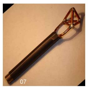
06-07. Slide a 2 ¾-inch piece of shrinkable tubing over the all-thread of the tetrahedral frame. It should leave about ¼-inch of thread at the bottom and cover the soldered junction of the pipe to the U-frame.
