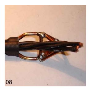
08. Align the 4 lengths of shielded wire so that the wire numbers are 2-1-3-4 clockwise. You should be able to push the wires through the tube from the bottom. The slight twist as shown in the picture is not usually necessary. Push the ends past the top of the tetrahedral and undo any twist you may have through the pipe by pulling all of the wires together back and forth while untwisting.
